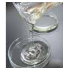
Adoption of Neopulim™ is advancing in information and communications field such as smartphone parts, taking advantage of the material's colorless transparency and heat resistance exceeding 300°C.
